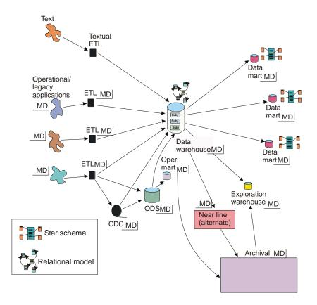
Fig 12 shows that in the center of the hub is the Inmon corporate information factory. In the Inmon corporate information factory is the "single version of the truth". The data here is granular, historical and integrated. The data here is cast in the form of the relational model.
